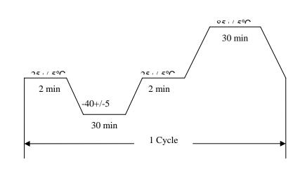
\*Frequency variation shall be within +/-5ppm and equivalent resistance less than ±15% max. after the test. Note: Measuring the frequency should be done after keeping test samples at room temperature for 24 hours.
